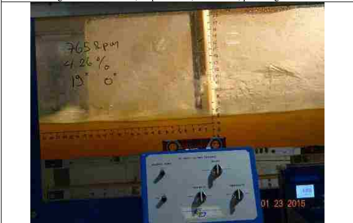
Figure 164. 765 RPM, slope: 4.26%, L_{bb}= 19'' , pitch angle = 0^\circ
