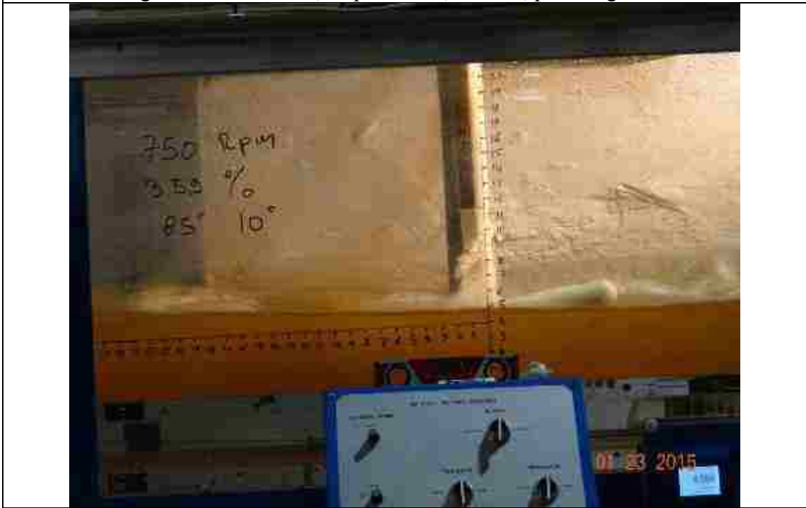
Figure 156. 750 RPM, slope: 3.59%, L_{bb}=8.5'' , pitch angle = 10^\circ
