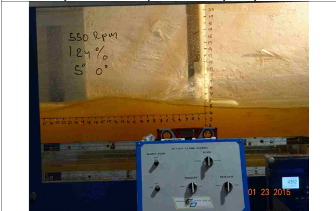
Figure 62. 550 RPM, slope: 1.24%, L_{bb}=5'' , pitch angle = 0^\circ
