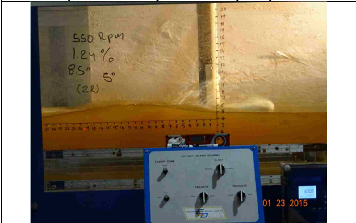
Figure 68. 550 RPM, slope: 1.24%, L_{bb}=8.5'' , pitch angle = 5^\circ
