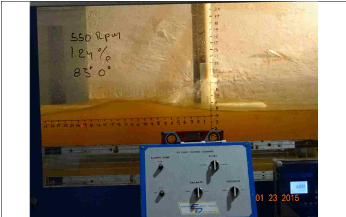
Figure 63. 550 RPM, slope: 1.24%, L_{bb}= 8.5'' , pitch angle = 0^\circ
