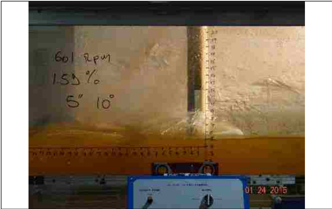
Figure 85. 601 RPM, slope: 1.59%, L_{bb}= 5'' , pitch angle = 10^\circ
