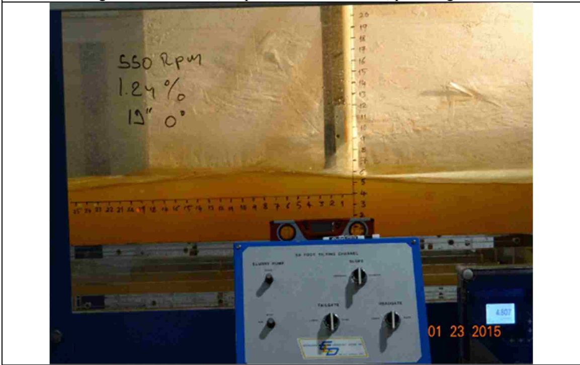
Figure 66. 550 RPM, slope: 1.24%, L_{bb}= 19'' , pitch angle = 0^\circ
