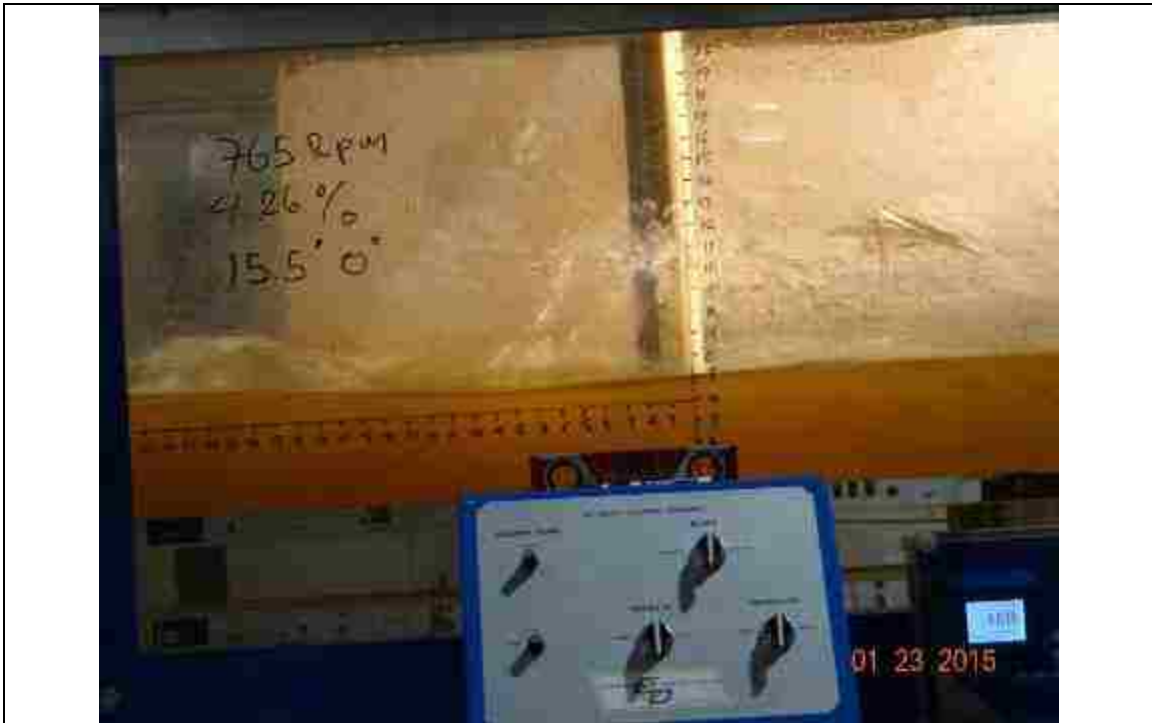
Figure 163. 765 RPM, slope: 4.26%, L_{bb}= 15.5'' , pitch angle = 0^\circ
