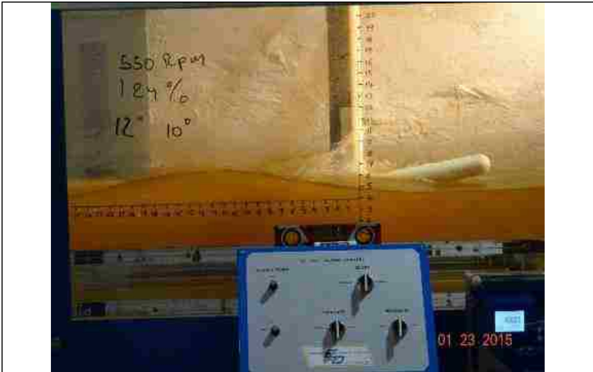
Figure 73. 550 RPM, slope: 1.24%, L_{bb}=12'' , pitch angle = 10^\circ
