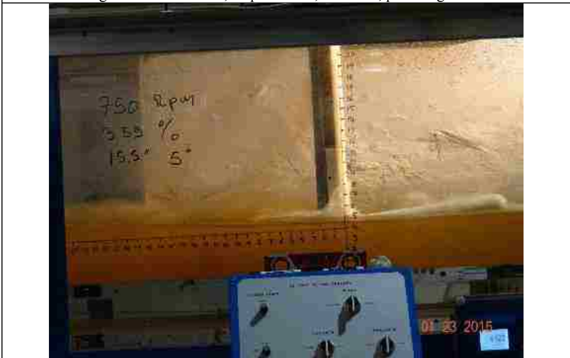
Figure 154. 750 RPM, slope: 3.59%, L_{bb}= 15.5'' , pitch angle = 5^\circ
