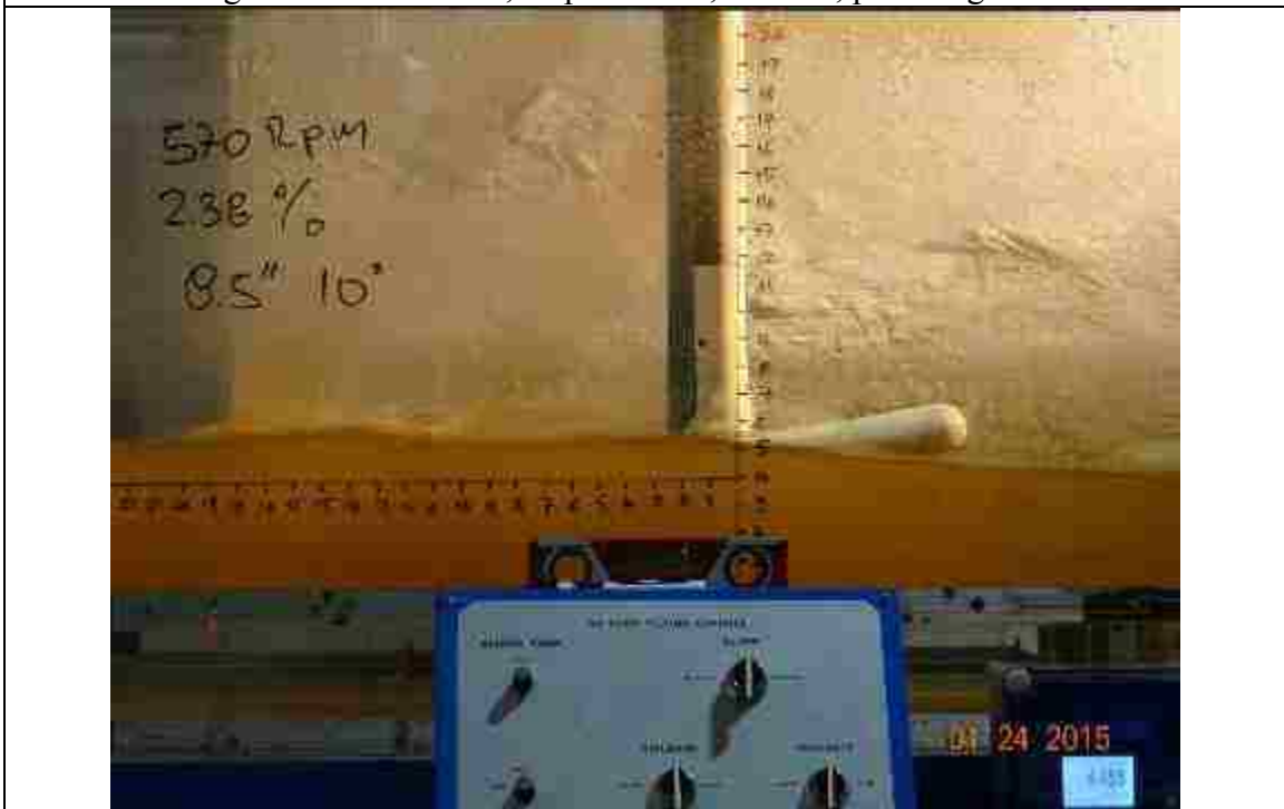
Figure 114. 570 RPM, slope: 2.38%, L_{bb}= 8.5'' , pitch angle = 10^\circ
