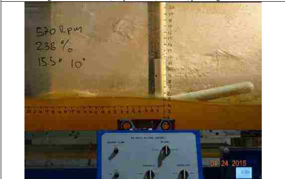
Figure 116. 570 RPM, slope: 2.38%, L_{bb}= 15.5'' , pitch angle = 10^\circ
