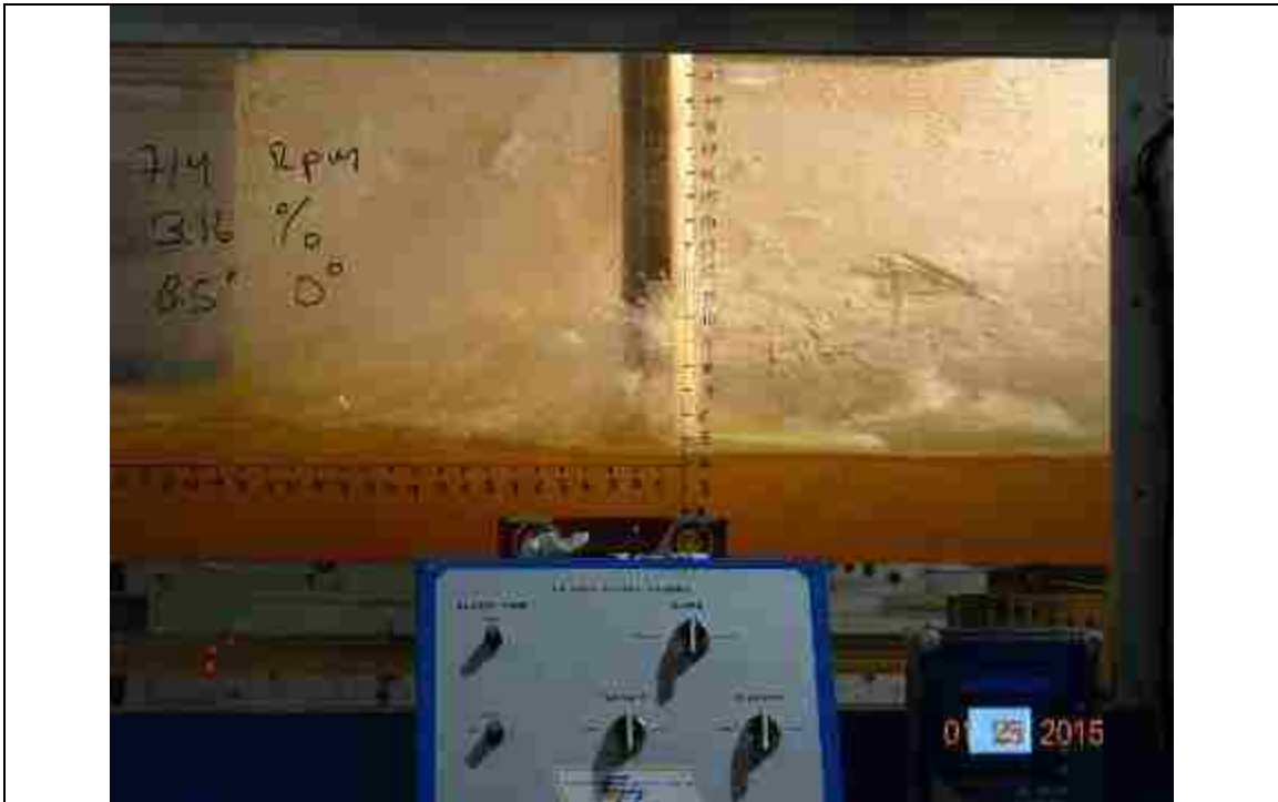
Figure 133. 714 RPM, slope: 3.16%, L_{bb} = 8.5'' , pitch angle = 0^\circ
