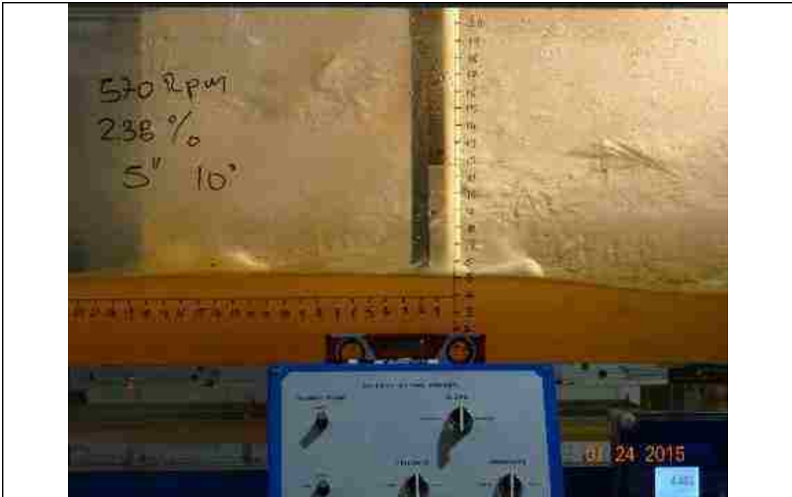
Figure 113. 570 RPM, slope: 2.38%, L_{bb}= 5'' , pitch angle = 10^\circ
