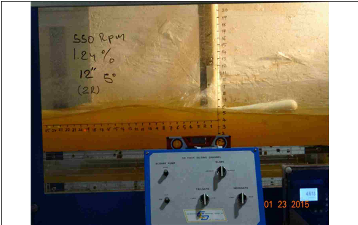
Figure 69. 550 RPM, slope: 1.24%, L_{bb}= 12'' , pitch angle = 5^\circ
