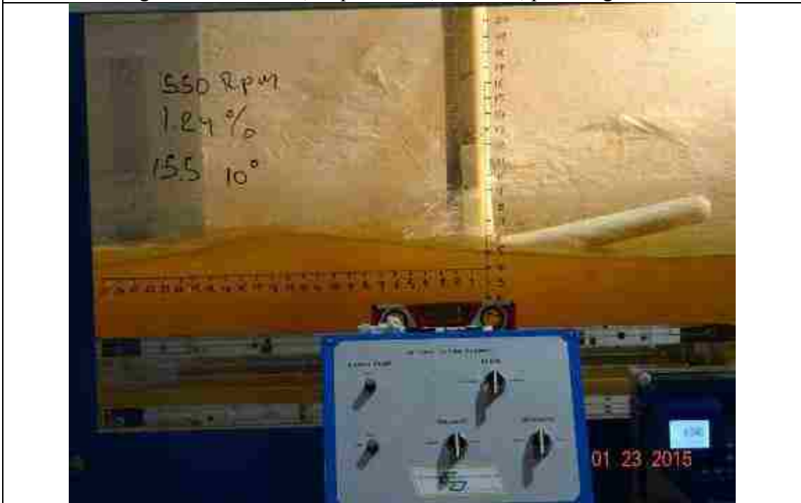
Figure 74. 550 RPM, slope: 1.24%, L_{bb}=15.5'' , pitch angle = 10^\circ
