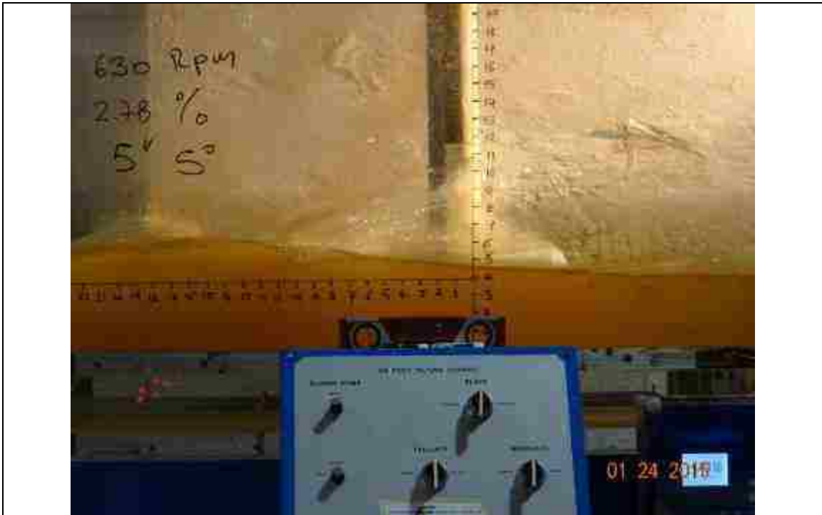
Figure 123. 630 RPM, slope: 2.78%, L_{bb}= 5'' , pitch angle = 5^\circ
