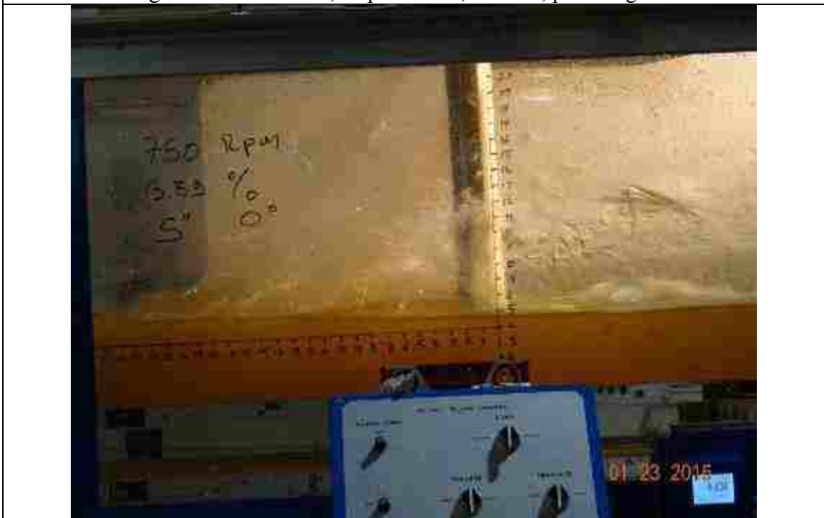
Figure 146. 750 RPM, slope: 3.59%, L_{bb} = 5'' , pitch angle = 0^\circ
