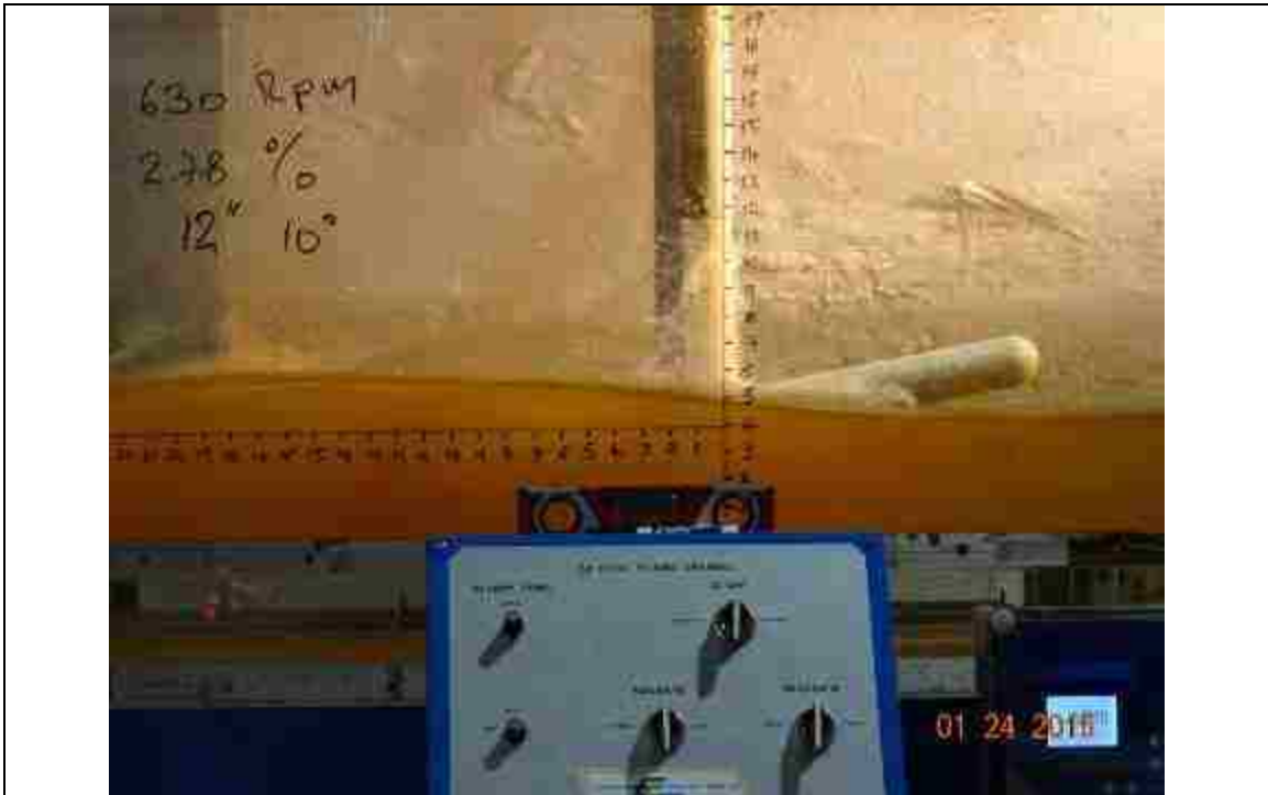
Figure 129. 630 RPM, slope: 2.78%, L_{bb} = 12'' , pitch angle = 10^\circ
