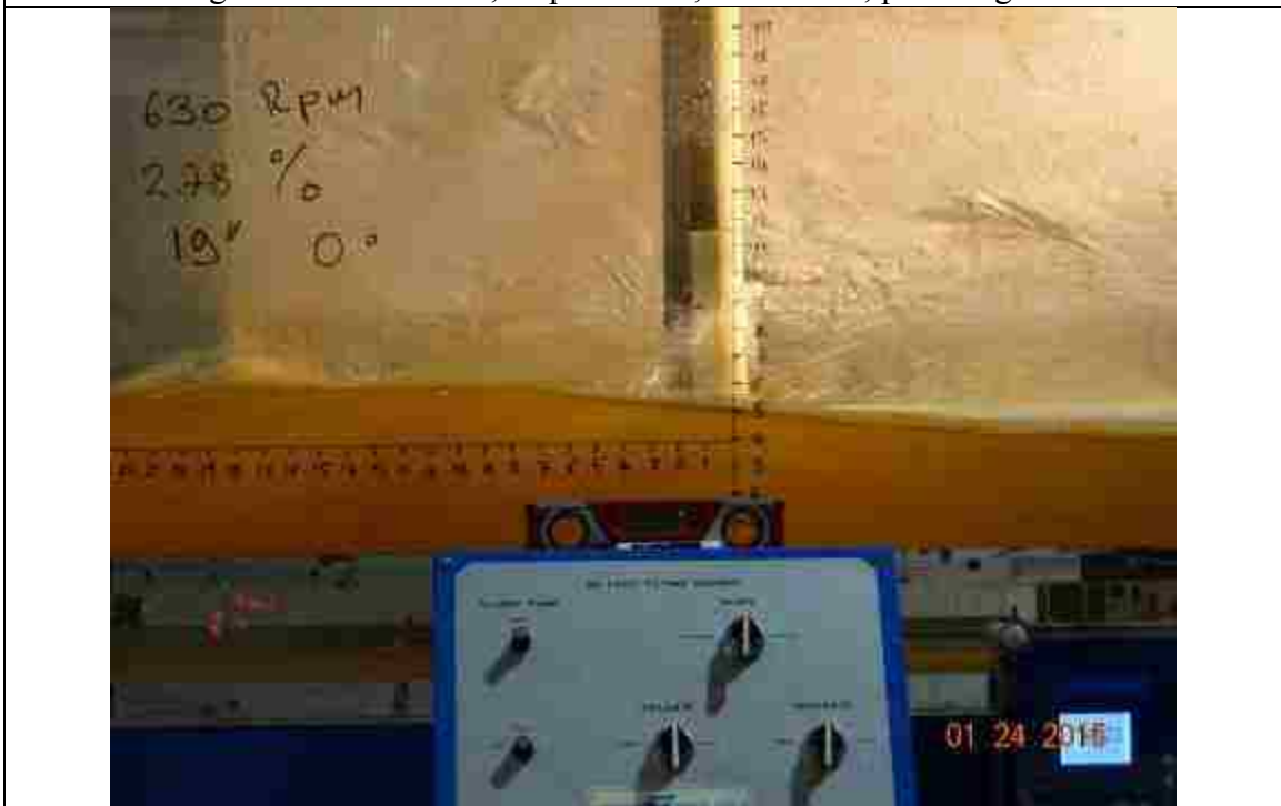
Figure 122. 630 RPM, slope: 2.78%, L_{bb}= 19'' , pitch angle = 0^\circ
