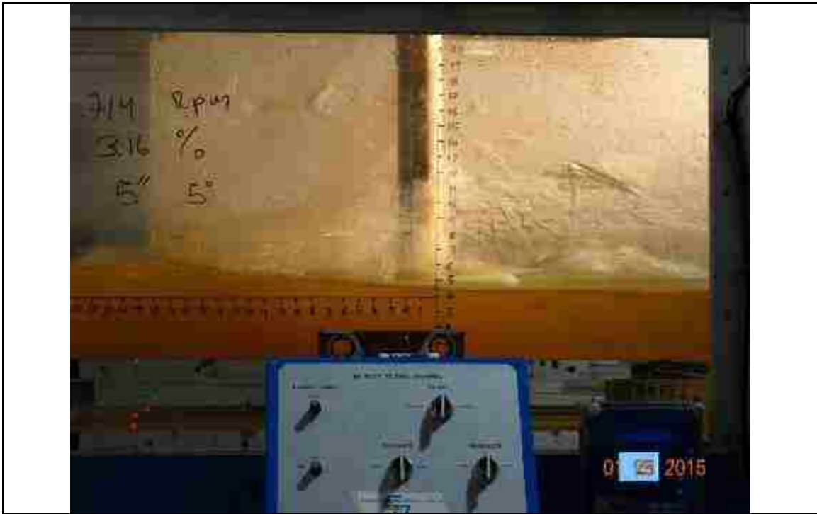
Figure 137. 714 RPM, slope: 3.16%, L_{bb}= 5'' , pitch angle = 5^\circ
