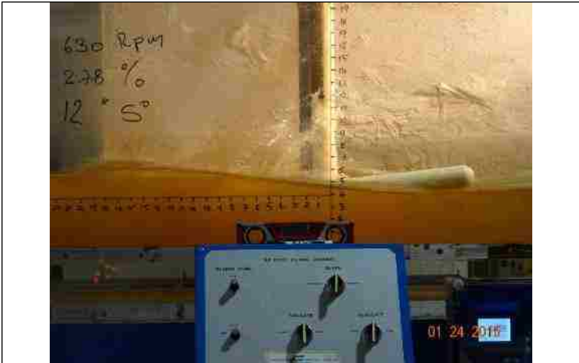
Figure 125. 630 RPM, slope: 2.78%, L_{bb} = 12'' , pitch angle = 5^\circ
