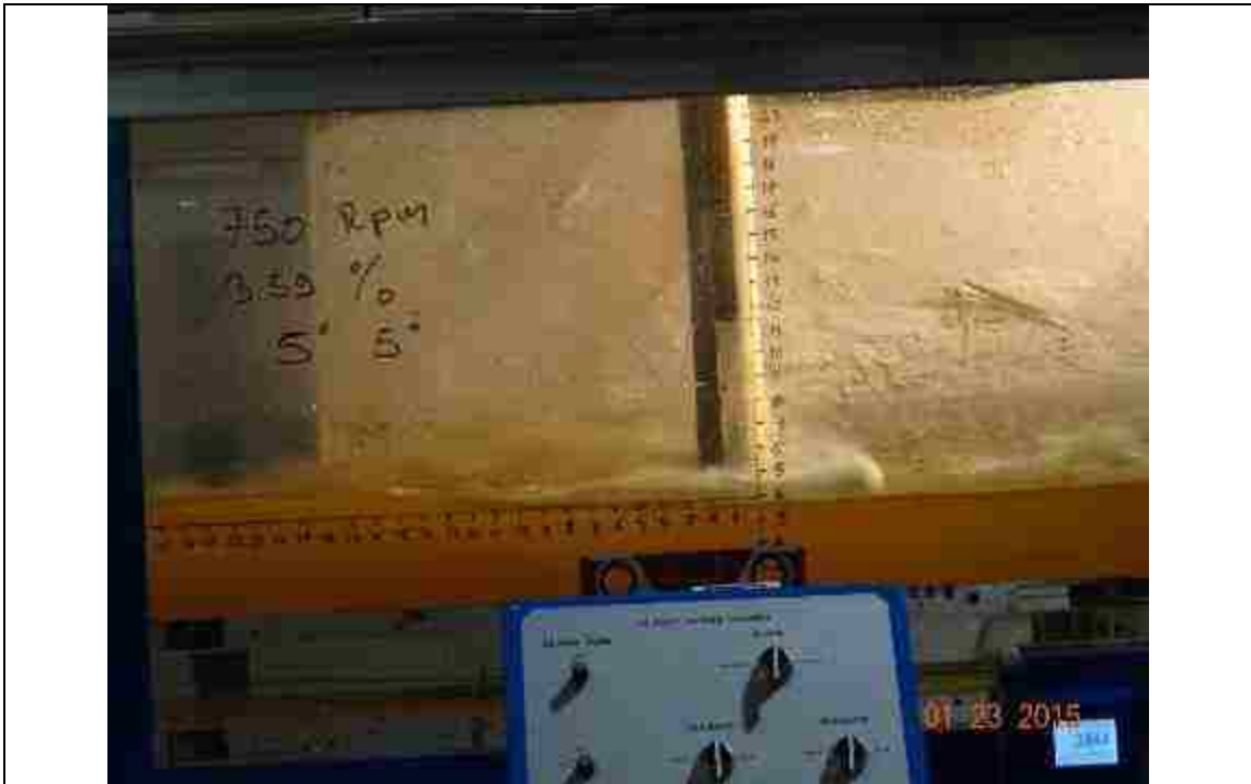
Figure 151. 750 RPM, slope: 3.59%, L_{bb} = 5'' , pitch angle = 5^\circ
