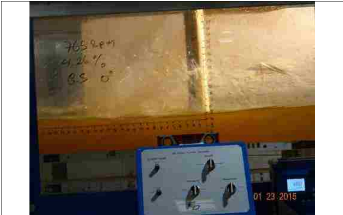
Figure 161. 765 RPM, slope: 4.26%, L_{bb} = 8.5'' , pitch angle = 0^\circ
