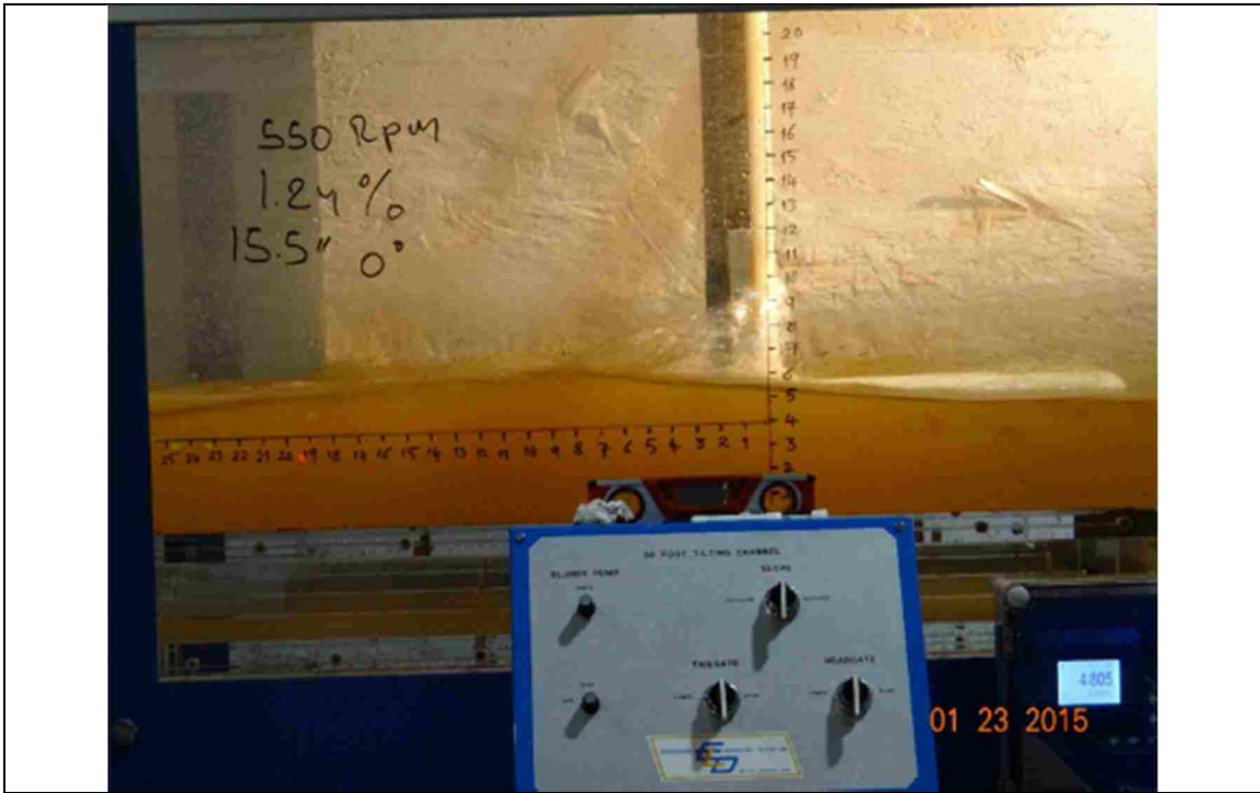
Figure 65. 550 RPM, slope: 1.24%, L_{bb}= 15.5'' , pitch angle = 0^\circ
