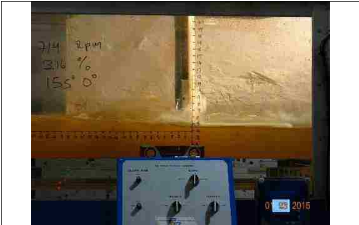
Figure 135. 714 RPM, slope: 3.16%, L_{bb}= 15.5'' , pitch angle = 0^\circ
