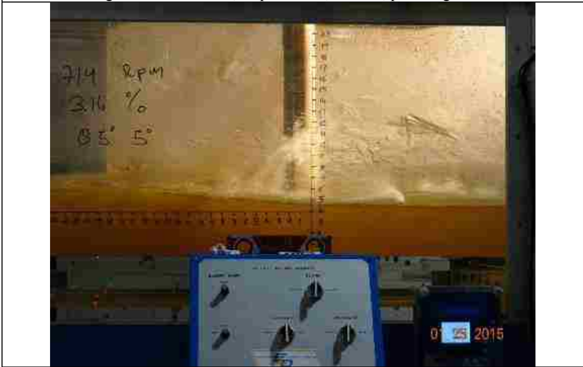
Figure 138. 714 RPM, slope: 3.16%, L_{bb}= 0'' , pitch angle = 5^\circ
