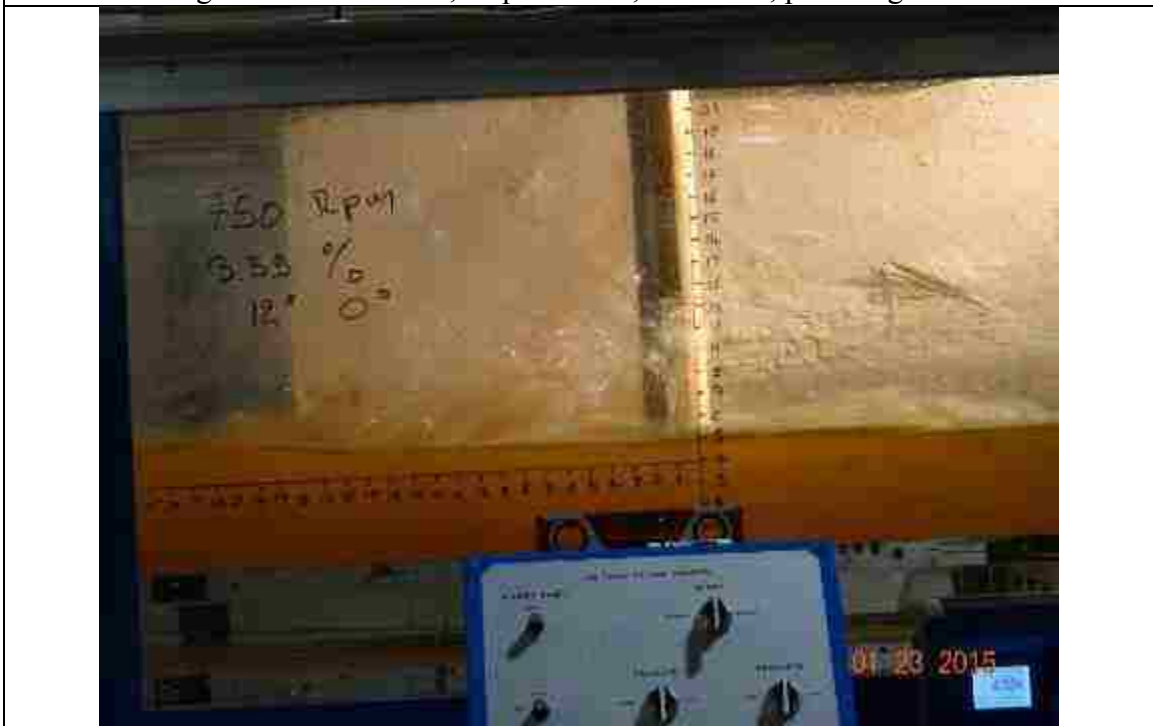
Figure 148. 750 RPM, slope: 3.59%, L_{bb} = 12'' , pitch angle = 0^\circ
