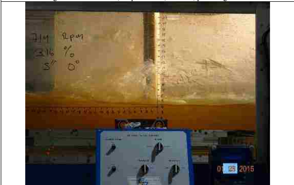
Figure 132. 714 RPM, slope: 3.16%, L_{bb} = 5'' , pitch angle = 0^\circ
