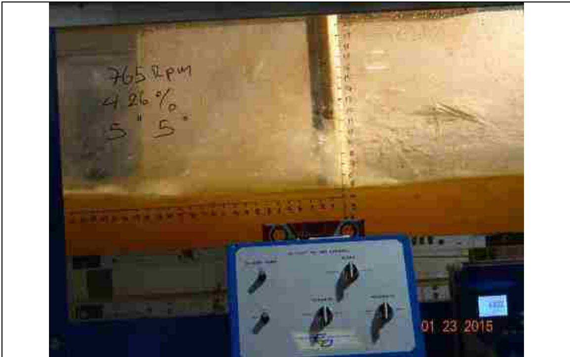
Figure 165. 765 RPM, slope: 4.26%, L_{bb}= 5'' , pitch angle = 5^\circ
