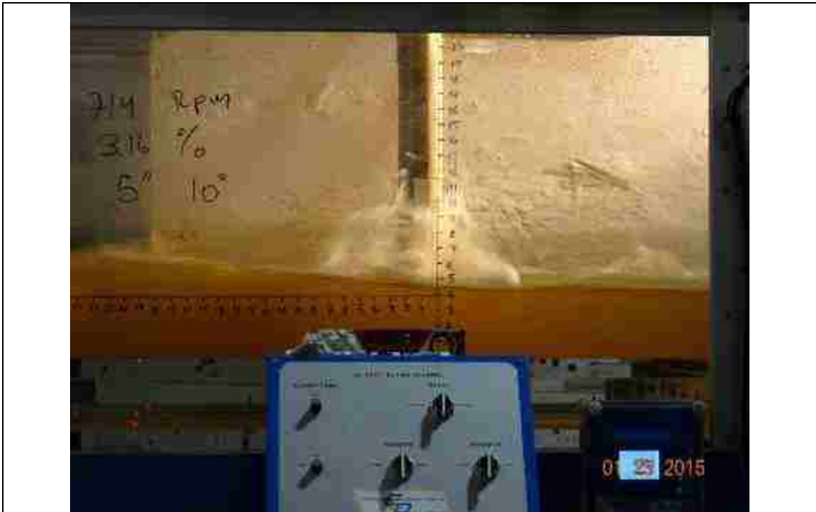
Figure 141. 714 RPM, slope: 3.16%, L_{bb}=5'' , pitch angle = 10^\circ
