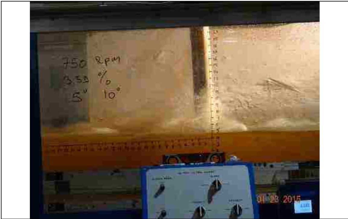
Figure 155. 750 RPM, slope: 3.59%, L_{bb}=5'' , pitch angle = 10^\circ
